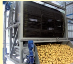
MACHINE TIPPING 2.5 TONNES BOXES
