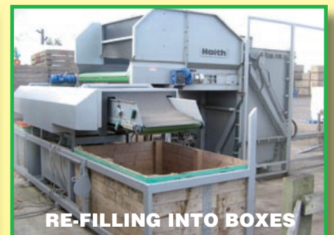
STORE HOLDING HOPPER
