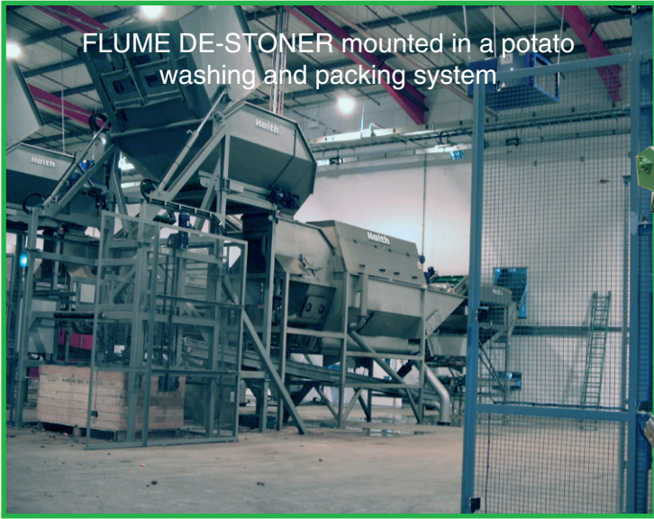
FLUME DE-STONER with auger in base tank for automatic sludge removal
