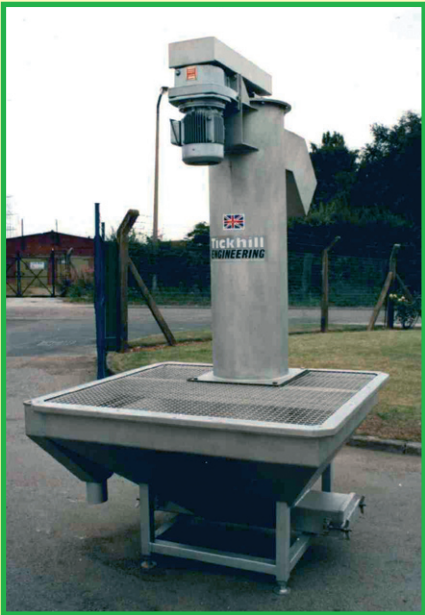
Wide in feed chute with water flume to assist product flow
