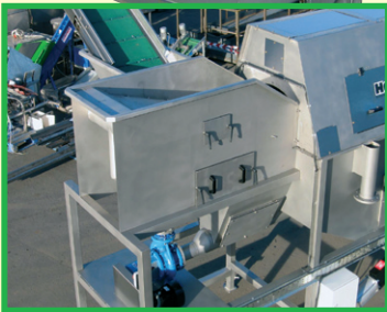
Flume de-stoner mounted on washer in feed
