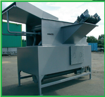
Wide in feed chute with water flume to assist product flow
