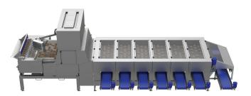
The **Celox P-UHD by Newtec** is an optical sorting machine available in 12 and 4 lane configurations. It simultaneously sorts by quality, size, and shape – elimnating the need for pre-grading.
